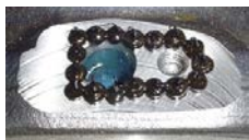
Grease extruded on brake part
