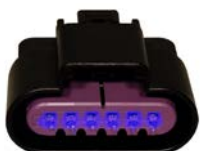
Greased connector shown with UV light
